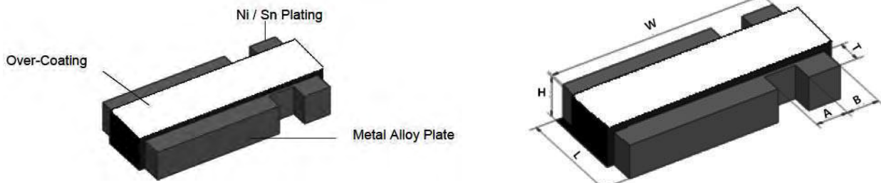
(LRF) Kelvin Current Sensing Chips Dimensions (Unit: mm)
