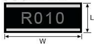
Current Detecting (CS) - Dimensions
