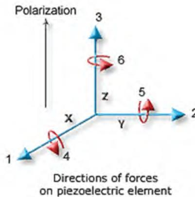
(Figure-1) - Directions of forces on piezoelectric element
