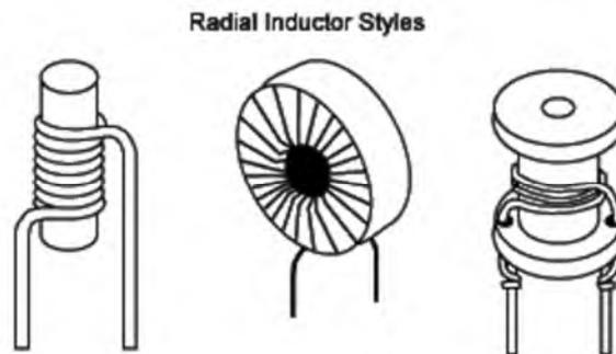
An inductor constructed on a core with leads exiting from the same side of the inductor body as to be mounted in the same plane. Radial inductors most often refer to two lead devices but technically include devices with more than two leads as well. Some common core shapes include rod cores, bobbins and toroid. (see Inductor)
