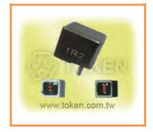
The Nickel Core Integrated Inductor (TCDY) measure high current rating up to DC 40 Amp., frequency high up to 1.0MHz with low DC resistance. Three compact sizes are available, 8.2mm x 8.2mm, 10.2mm x 10.2mm, and 12.5mm x 12.5mm. Making them ideally for today's DC/DC converter in distributed power systems or VRM, and motherboards for laptop and desktop computers applications.
