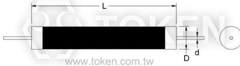
Ultra-Precision High Voltage Resistor Unpainted Dimensions (Unit: mm) - (HI80T)
