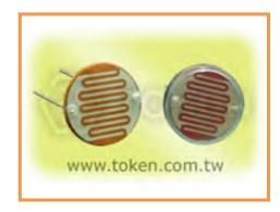
The photo-resistor, CdS, or LDR finds many uses as a low cost photo sensitive element and was used for many years in photographic light meters as well as in other applications such as smoke, flame and burglar detectors, card readers and lighting controls for street lamps.
