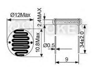
Epoxy resin package 12mm Cds PGM12\*\* series Dimensions (Unit: mm)
