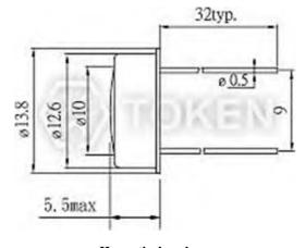
Hermetical package 12mm Cds PGM12\*\*-MP series Dimensions (Unit: mm)
