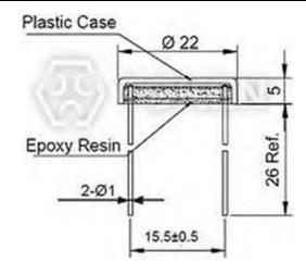
Hermetical package 20mm CdS PGM20\*\*-PP series Dimensions (Unit: mm)
