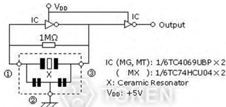
MHz (ZTT) Test Circuit for MOS IC
