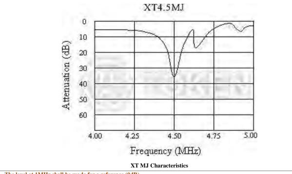
• The level at 1MHz shall be made for a reference (0dB).
