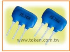
Token Double Trap Filter (XT MW) Series consist of 2 wafers with 2 trap frequencies. Recommended for Multi standard set. Features with good performance of attenuation and space saving with 3-terminal type. The characteristic of a three-terminal ceramic trap equals two two-terminal ceramic traps. Three-terminal ceramic trap has a monolith structure formed from 2 ceramic resonators.
