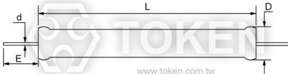
Ultra-Precision High Voltage Resistor Unpainted Dimensions (Unit: mm) - (HI80T)
