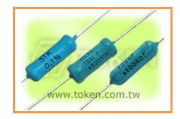
The resistance element in these devices is a precisely controlled thin film of metal alloy deposited on a high quality alumina substrate. Plated caps are force-fitted before the assembly is trimmed using advanced laser techniques to ensure excellent performance and low electrical noise. Leads are welded to the end caps prior to the resistor being coated with epoxy.
