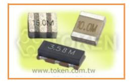
Token ZTAC and ZTTC series are the SMD ceramic resonators that meet the frequency tolerance  $\pm 0.5\%$ , temperature tolerance  $\pm 0.3\% \sim \pm 0.4\%$ , and aging tolerance  $\pm 0.3\%$ . The ZTAC and ZTTC covers the frequency range of 1.79 MHz to 50.00 MHz. ZTTC series features a built-in load capacitance. This feature eliminates any need for external loading capacitors and reduces component count, increases reliability and reduces size.
