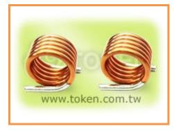
TRAD's inductance is unaffected by the current it carries. This contrasts with the situation with coils using ferromagnetic cores whose inductance tends to reach a peak at moderate field strengths before dropping towards zero as saturation approaches. (TRAD) series features better Q-factor, greater efficiency, greater power handling, highest possible SRFs, and less distortion.
